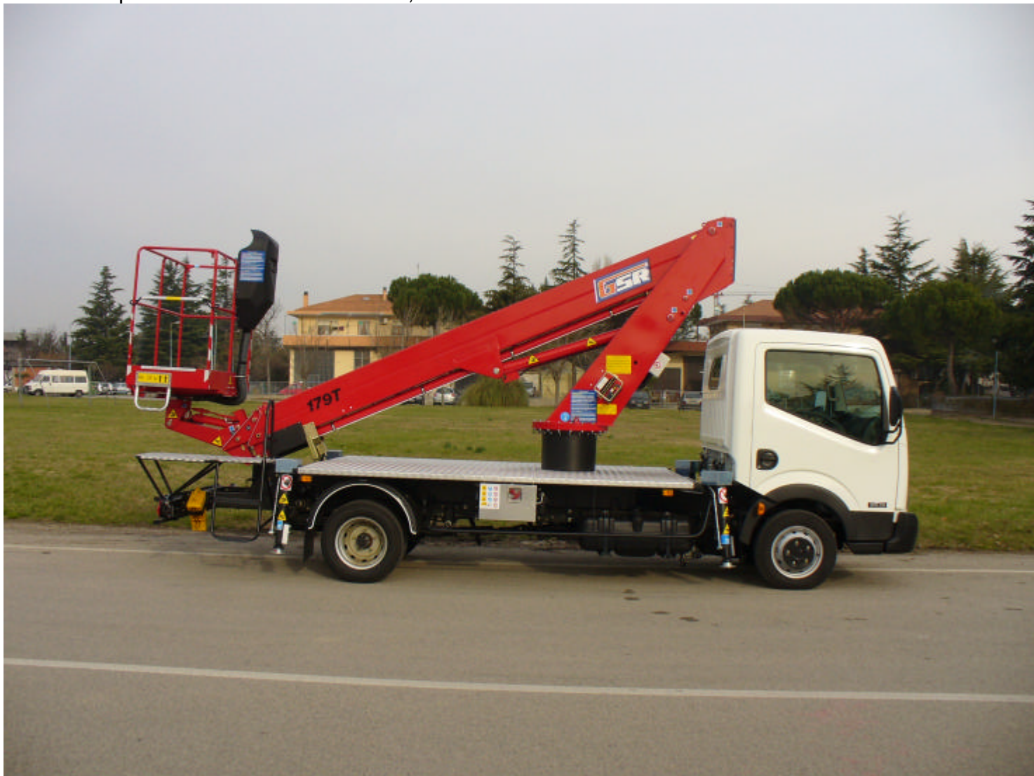
E179T compact VV on Nissan Cabstar 3,5T wheelbase 3400
