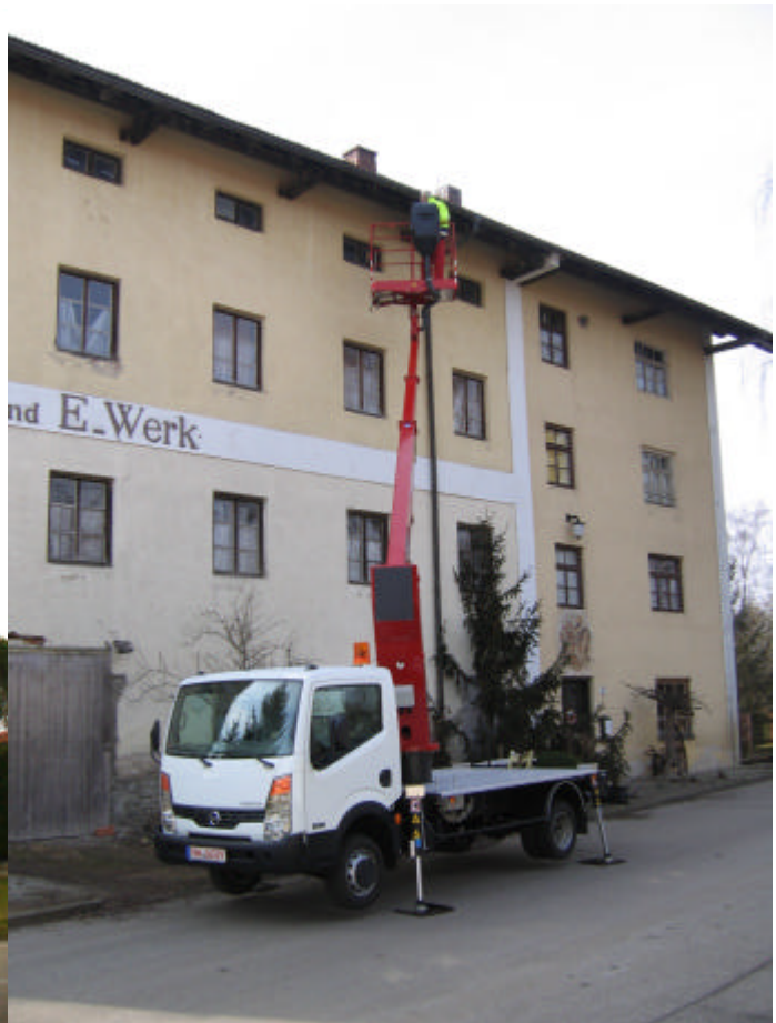
The E179T's light but rigid structure allows the operator to work in full comfort even at the maximum height/outreach angle.
